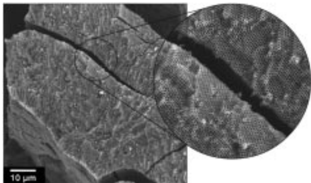
Figure 3. SEM of a macroporous \text{TiO}_2 crystal (anatase) with voids ordered over tens of micrometers ( 110 \times 60 \times 50 \mu\text{m} ).
